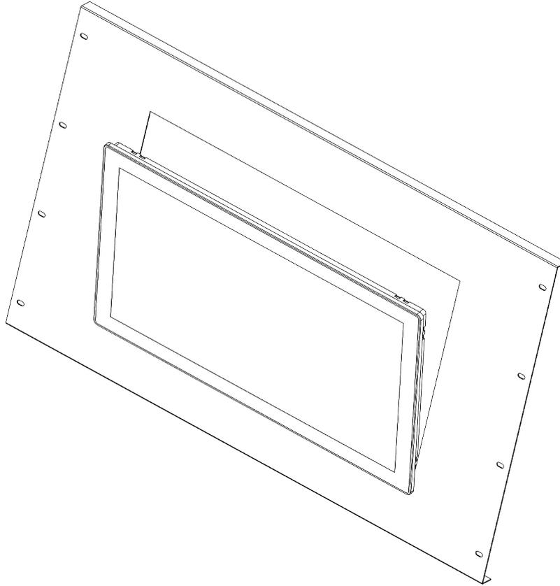
(2) Install the snaps into the side snap holes of the industrial all-in-one machine and then tighten the screws as shown in the figure below;
