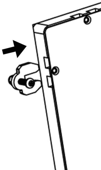
(3) The installed interface is shown in the figure below. The installation of the remaining snaps is similar to this operation.
