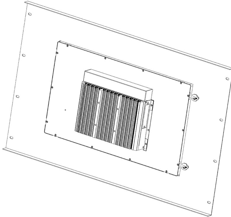
Note: The installation of snaps for PPC-C1227/C1527/C1627 requires 4 pieces. The installation of snaps for PPC-C1727/C1827/C2127 requires 8 pieces.
